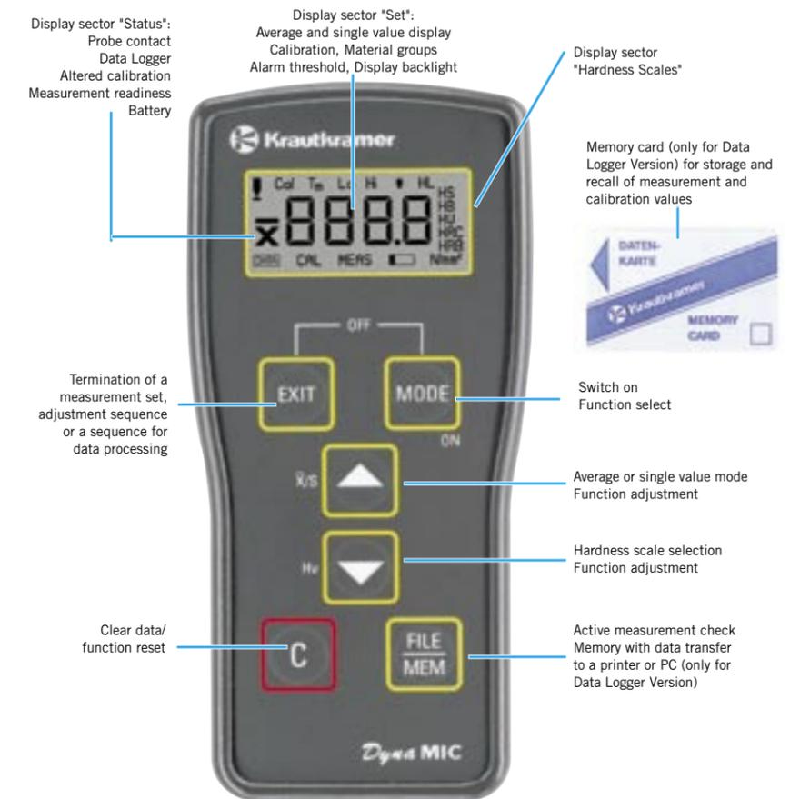
The DynaMIC also ensures measurement reliability by displaying the total number of all measurements taken with an impact device. This assists in scheduling maintenance or predicting replacement of the impact body.
