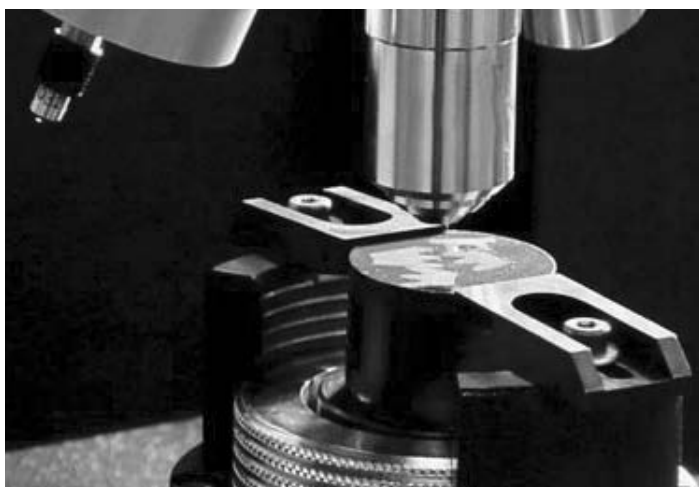
Microindentation testing of gear teeth
