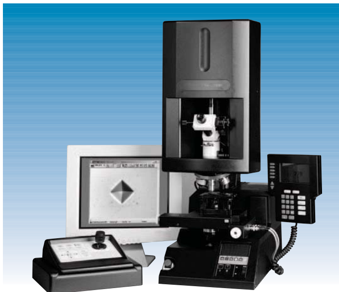
Wilson Instruments series T2100 Knoop/ Vickers tester with ATA premium fully automatic XY auto traversing system
