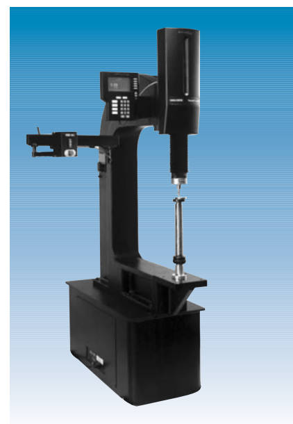
Modified Rockwell 2000 with Brinell test frame to accommodate testing of extremely large parts
