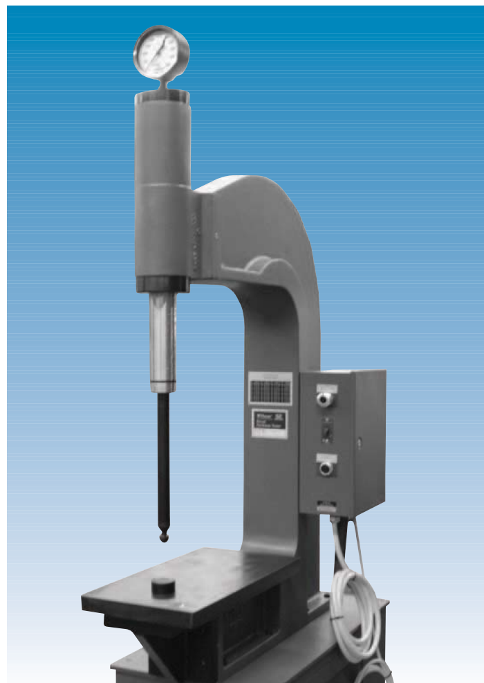
Wilson Brinell Model AP shown with removable ram extension to test small parts
