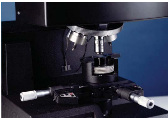
Sample mounted in UCL for testing, using x-y stage with digital micrometers
