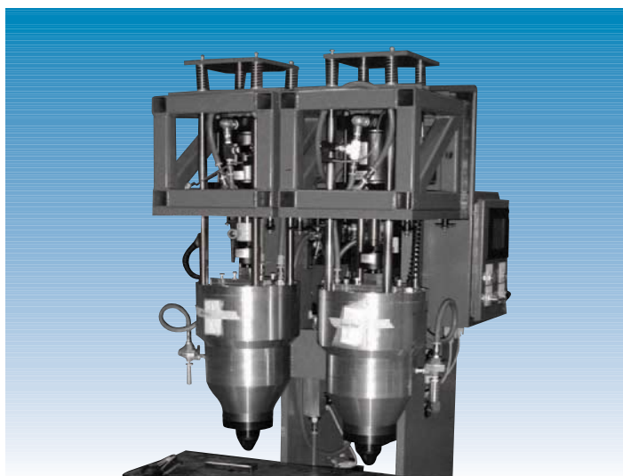
Custom-designed dual head production Brinell
