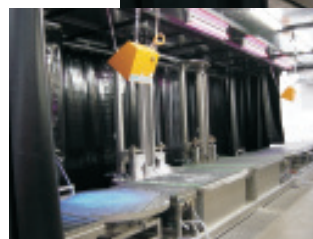
State-of-the-art penetrant systems including drying furnace to test aircraft part
